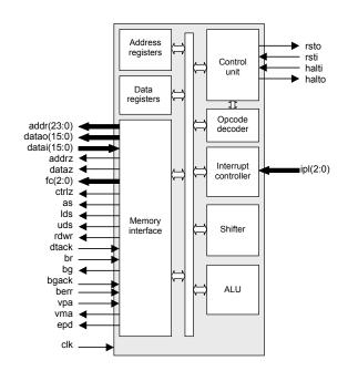
**Control Unit** – Performs the core synchronization and data flow control. This module manages execution of all instructions. Contains SR (status register is consisted of two portions supervisor byte and user byte) and its related logic.
